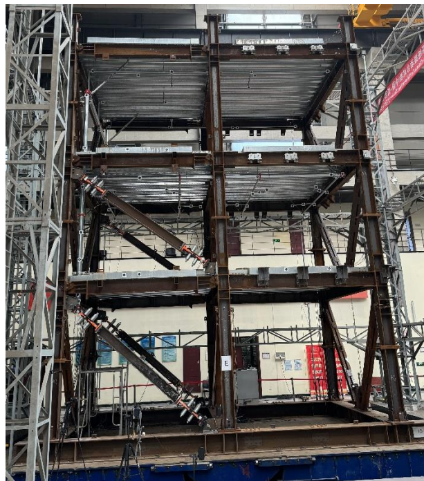
Figure 3: RSFJ tension-compression configuration and brace structure.
