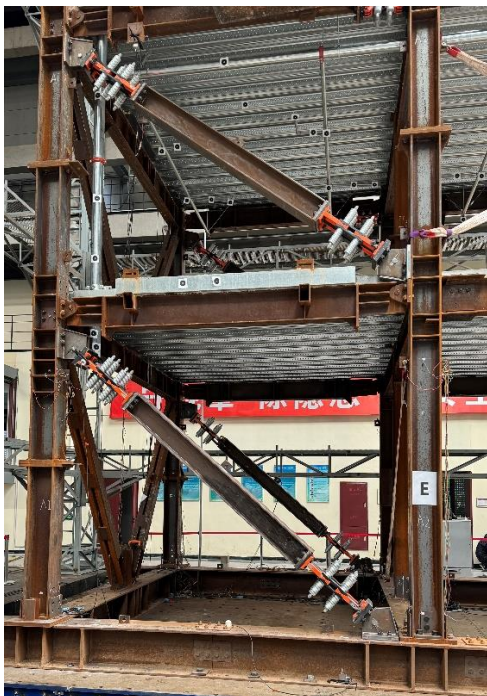
Figure 3: RSFJ tension-compression configuration and brace structure.
