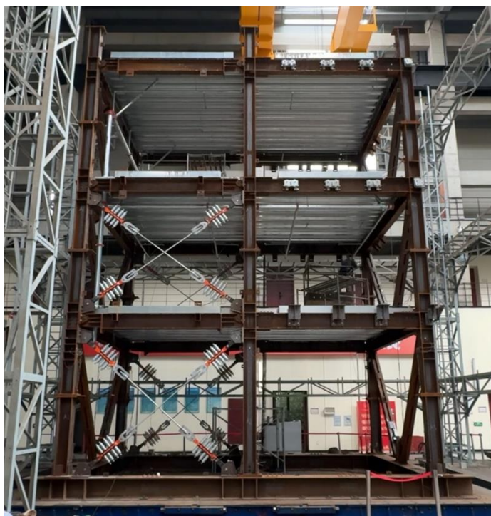
Figure 4: RSFJ tension-only configuration and brace structure.
